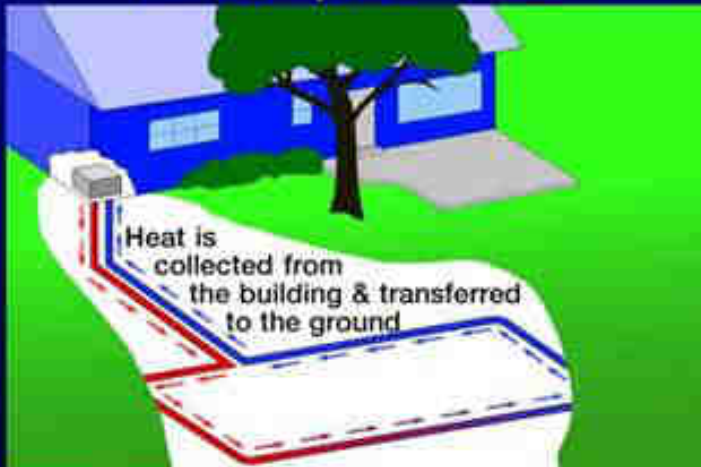
Heat Pump in Summer
